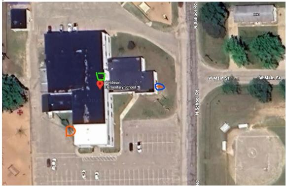
Mecosta: The current DMARC is a tower designated as a red circle, and the green box is the MDF. The desired DMARC point for this project is designated below by a red line and blue circle, near W. Main Street.
