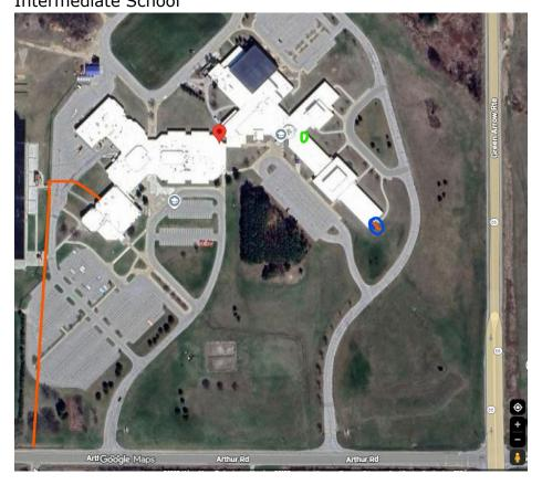
Weidman: The red circle is the school's current tower, and the green box is the MDF. Ideally, keeping it out at N School Road is preferred to prevent the disturbance of the existing pavement. The desired demarcation (DMARC) point is the red line with the blue circle.
