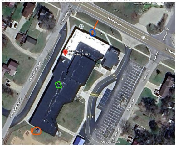
Barryton: The current DMARC is a tower designated as a red circle, and the green box is the MDF. The desired DMARC point for this project is designated by a red line and blue circle, near M66.
